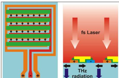
**Tera-SED** functional principle: with applied bias voltage the electric field direction is reversed between successive electrode fingers. An optically opaque metal layer is applied between every other finger pair such that optical excitation is only possible in areas exhibiting the same electric field direction. THz radiation emitted from the device thus interferes constructively in the far-field.
