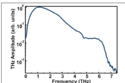
**Tera-SED3** emission spectrum at 10 V DC bias and 0.7 nj pulse energy, acquired with Laser Quantum GmbH (formerly Gigaoptics) ' High-Speed ASOPS technique.
