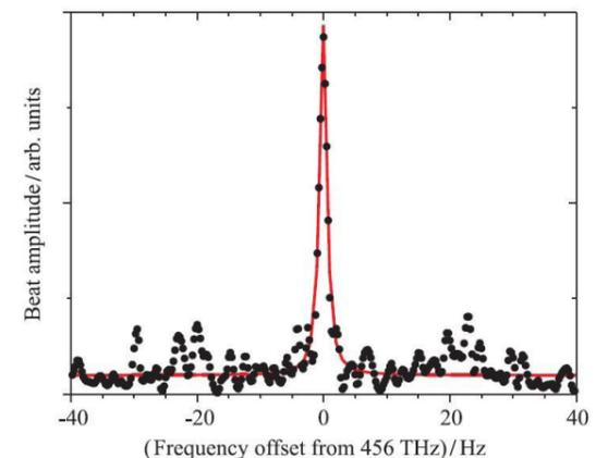
Figure 3: Heterodyne beat between two ultrastable cw lasers at 532 THz and at 456 THz via a Laser Quantum 1 GHz Ti:Sapphire laser recorded at the U.S. National Institute of Standards and Technology.
