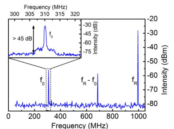
Figure 4: Carrier-envelope offset beat obtained from the **taccor comb**. The signal-to-noise ratio is limited by the RF spectrum analyzer. The close-up in the inset reveals the true signal-to-noise ratio of >40 dB in 100 kHz of bandwidth.
