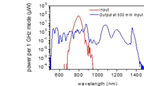
Figure 2: Red: Typical **taccor** output spectrum used for CEO detection and comb applications. Blue: Output spectrum after 1 m photonic crystal fiber.
