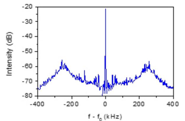
Figure 6: Close-up of the phase-locked  $f_{\text{CEO}}$ . The data is acquired using a resolution bandwidth of 200 Hz. The servo bandwidth is about 250 kHz as indicated by the symmetrical peaks around the carrier.
