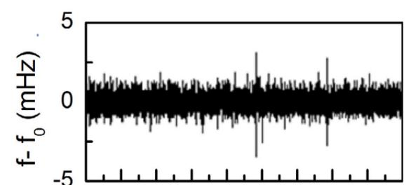
Figure 7: Long term deviations from the lock point of a CEO beat stabilised at 310 MHz over 25 h showing exceptional stability (limited by RF reference input).
