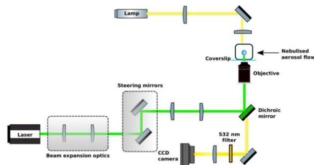
Figure 2: Optical Tweezer set up
