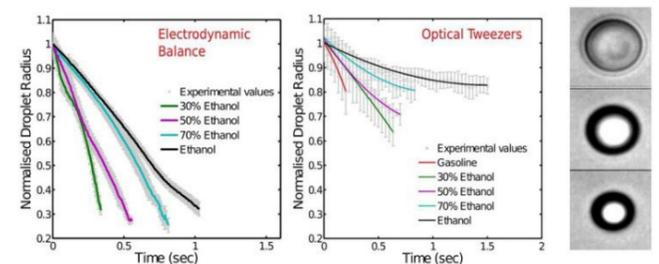
Figure 3: Evaporation trends of ethanol/gasoline droplets trapped by Electrodynamic Balance (a) and Optical Tweezers
