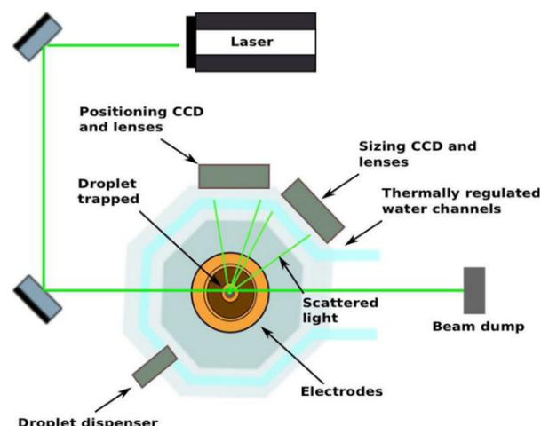
Figure 1: Electrodynamic Balance set up
