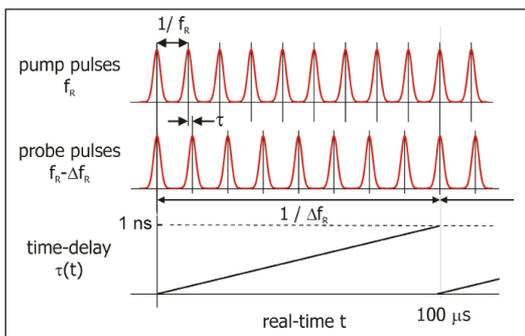
The **TL-1000-ASOPS** controls the time delay between pump and probe pulses by slightly differing repetition rates ( $f_r \sim 1$  GHz). The difference in  $\Delta f_r$  determines the scan rate, while the measurement window is given by the inverse of the repetition rate  $1/f_r = 1$  ns. Here,  $\Delta f_r$  is 10 kHz, i.e. the time-delay is repetitively ramped with a 100  $\mu$ s period.
